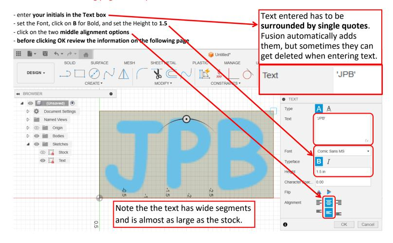
A key consideration is to have the text as large as possible while still maintaining about 0.1" between the edge of the stock and any text elements. It is also important to use text that doesn't have any narrow sections. All this will help ensure that the 1/8" endmill can mill out all the letters.
