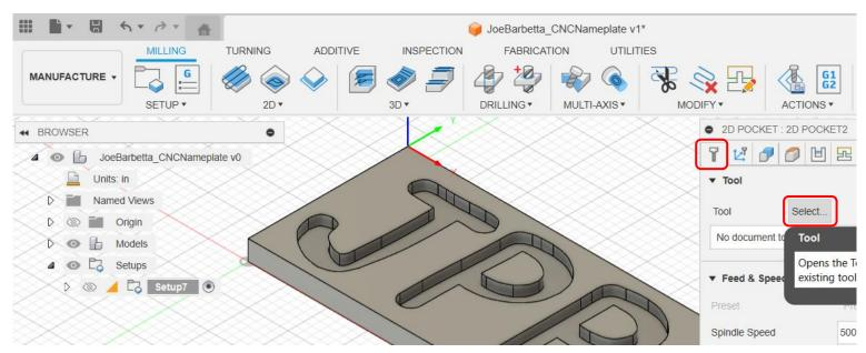
The tool typically used for milling is an end mill. It's flutes make it resemble a drill bit with a flat end and the flutes are formed so that it can cut sideways. A drill bit can only drill down into material, but it can't cut sideways. Most endmills are flat (no point at its end), but some do have a point, ball end, or other styles.
